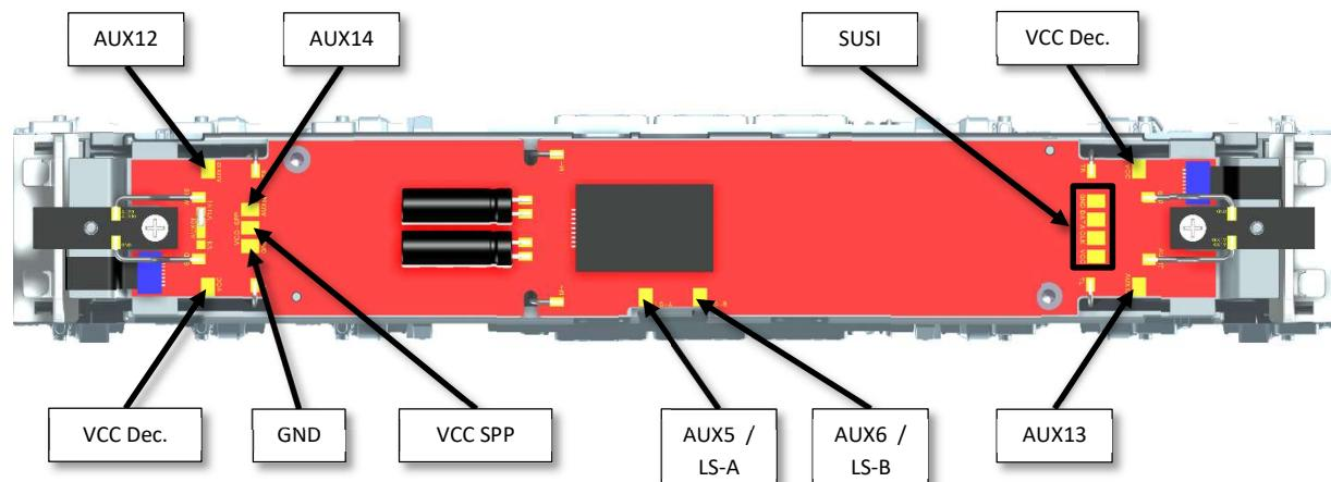
**Important!** VCC SPP = continuous positive voltage buffered, 8,2 Volt
