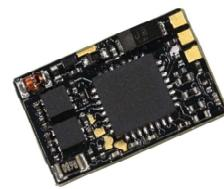
For Plug and Play you can use our **decoder item no. 66039** (train-O-matic). The decoder is completely programmed to use all functions of this modell (*excepting sound*).
